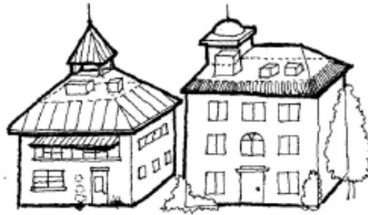
Figure 29. Examples of Screening Mechanical Equipment
